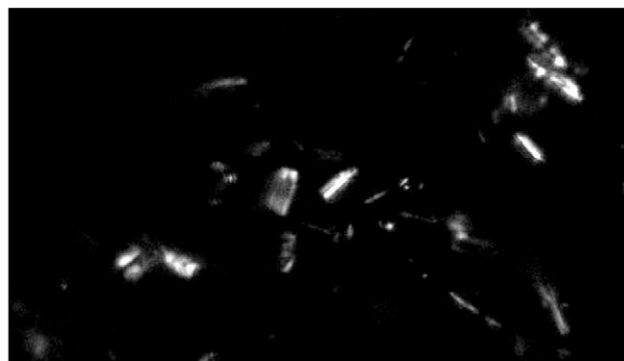
Fig. 3. Optically-active microfibril produced from gelatinized ae 70 HAS at slow (0.1 °C/min) cooling rate (image size 100 \times 180 \mu\text{m}^2 ).
